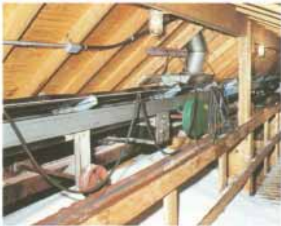
SHUTTLE-BELT CONVEYOR Under-slung drive, tri-roller idlers, bi-directional, up to 250 tph.
