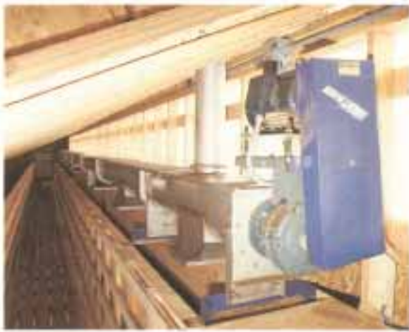
SCREW CONVEYOR Fully enclosed, 12", 14" or 16" dia. auger, up to 120 tph.
