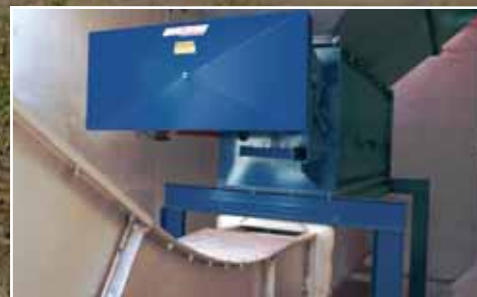
Easy-to-access material conditioner mounted below hopper.
