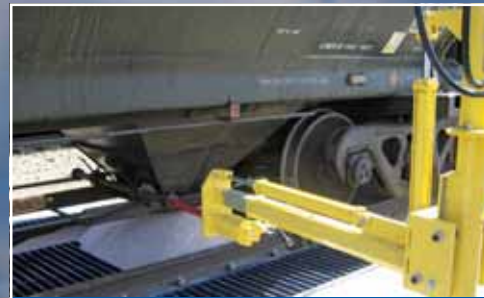
Railcar gate opener & large-volume rail hopper
