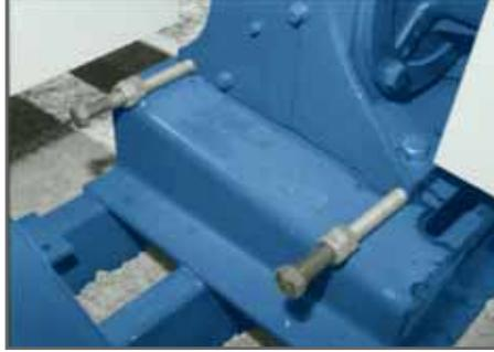
Exclusive: Two simple stainless steel screw shafts move the entire motor mount unit when adjusting drum drive chain tension. Drive chain can be adjusted independently of V-belts — so adjusting one does not require adjusting the other. For added insurance, Waconia's gearbox is extra heavy duty — designed for three times more horsepower.
